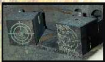
Standard Sensor — Failed due to weld slag adhesion after 1,663 Weld Cycles
