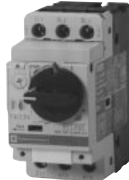
GV2P 0.1 to 25 A Up to 15 hp @ 460 V 50 kA withstand @ 480 V Rotary Handle Operator Visible Trip Indication
